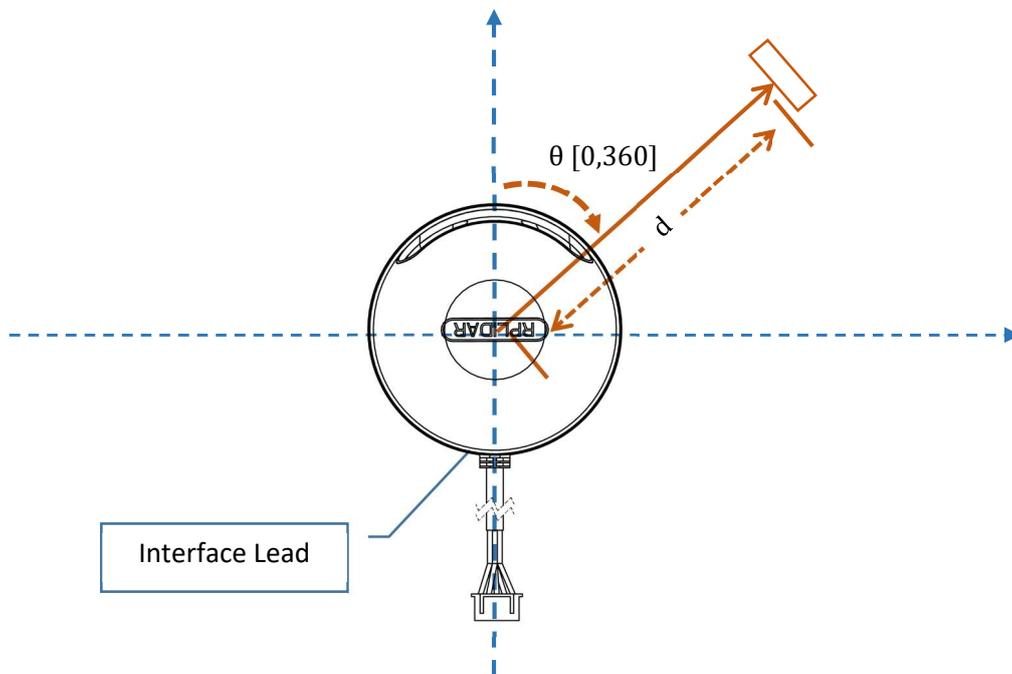
Figure 2-4 RPLIDAR Scanning Data Coordinate System Definition
