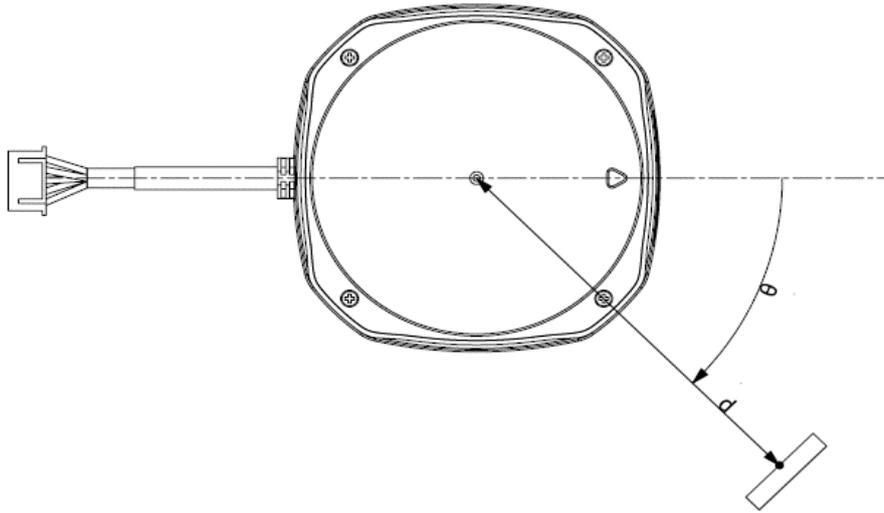
Figure 1-2 The RPLIDAR S2 Working Schematic
