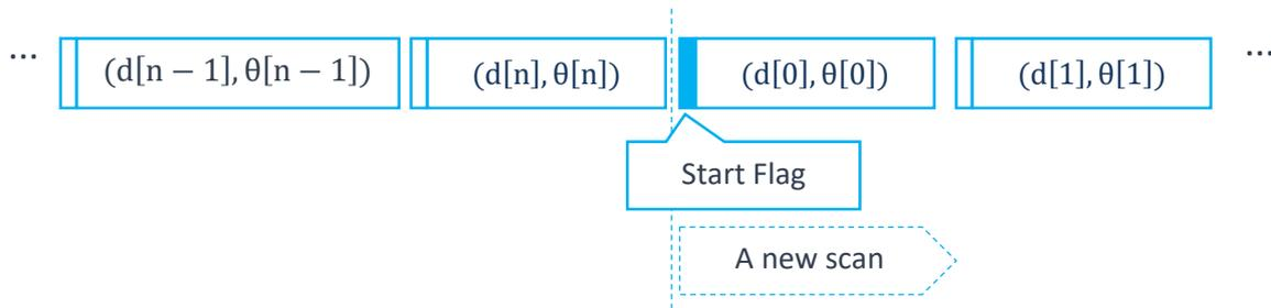
Figure 1-5 The RPLIDAR Sample Point Data Frames
