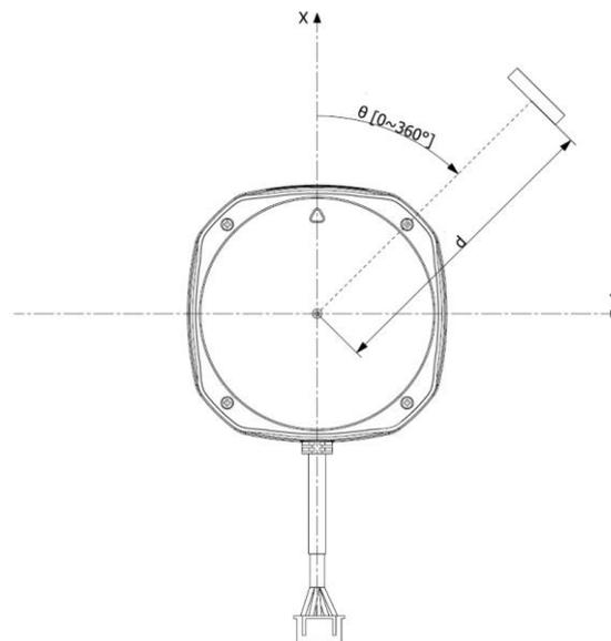
Figure 2-4 RPLIDAR S2 Scanning Data Coordinate System Definition
