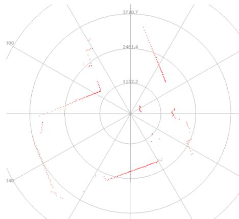
Figure 1-3 The Environment Map Obtained from RPLIDAR Scanning
