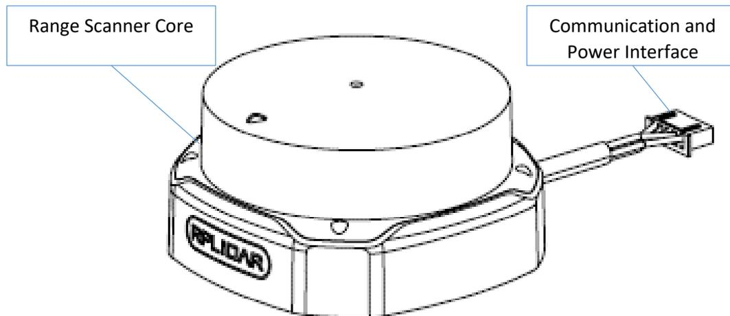
*Figure 1-1 RPLIDAR S2 System Composition*
