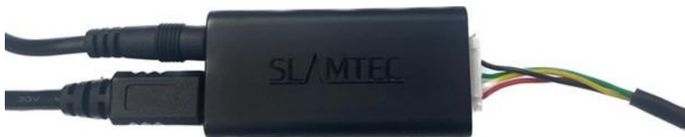
Figure 2-2 Connect the USB Adapter to PC via Micro-USB Cable
