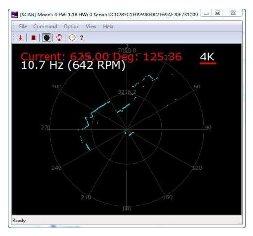
Figure 2-9 The Scan Outline in RPLIDAR Demo Application
