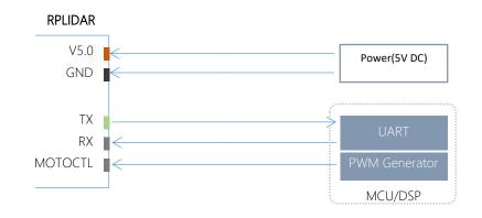
Figure 3-3 RPLIDAR A2 Pins Reference Design
