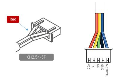
Figure 3-1 RPLIDAR A2 Pins
