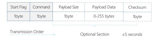
Figure 2-4 RPLIDAR Request Packets' Format
