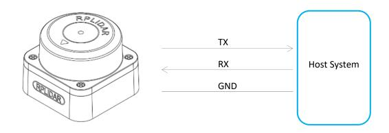
Figure 1-1 The Communication Between RPLIDAR and Host System
