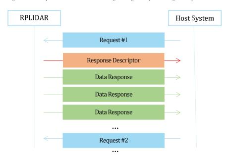
Figure 2-6 Response Packets Sent during a Single Request-Multiple Response Mode
