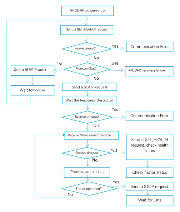
Figure 5-1 Recommendation for Starting RPLIDAR Scanning and Data Retrieving
