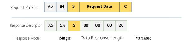
Use this command to fetch characters of RPLIDAR. Use type and payload to specify the configuration entry to query.
