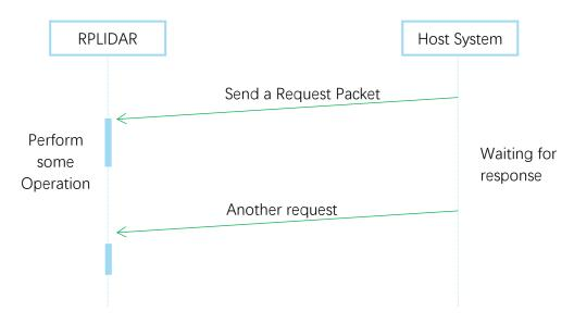
Figure 2-3 RPLIDAR Single Request-No Response Mode
