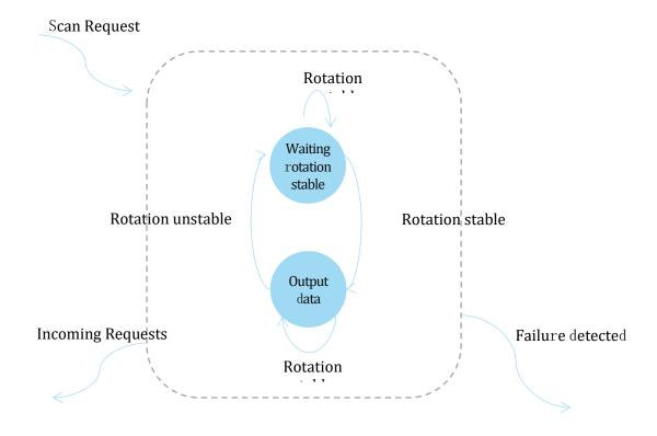
Figure 3-2 RPLIDAR's Working Mode during Scanning
