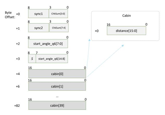
Figure 4-13 Format of a RPLIDAR Express Scan Data Response Packet (Dense Mode)
