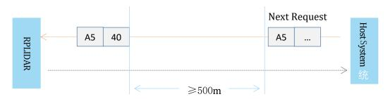
Figure 4-3 The Timing Sequence of a RESET Request
