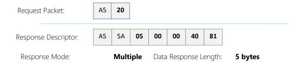
RPLIDAR, except for the RPLIDAR that is in the Protection Stop State, will enter the scanning state once it receives this request from a host system. Each measurement sample result will be sent out using an individual data response packet. If the RPLIDAR has been in scanning state already, it will stop the current measurement sampling and start a new round of scanning. This request will be ignored when RPLIDAR is in the Protection Stop state.
