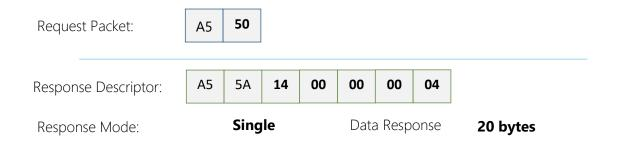
RPLIDAR will send out its device information (e.g. serial number, firmware/hardware version) to the host system once it receives this request.
