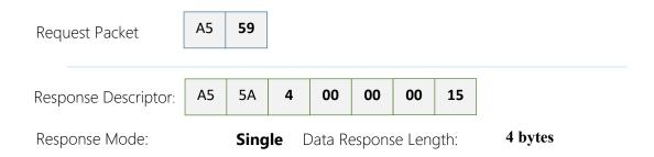
By sending this request, the host system can get the single measurement duration in standard scan mode and express scan mode respectively and calculate the current rotating speed of RPLIDAR accurately.
