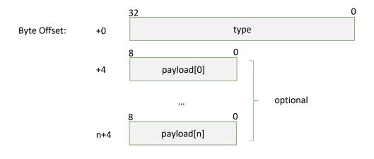
Figure 4-25 Format of a Get LIDAR Conf Request Packet
