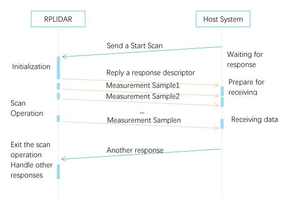
Figure 2-2 RPLIDAR Single Request - Multiple Response Mode
