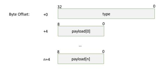
Figure 4-27 Format of a Get LIDAR Conf Response Packet
