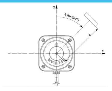
Figure 4-9 Angle and Distance Value Geometric Definition for RPLIDAR C1 series
