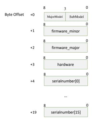
Figure 4-18 Format of a Device Info Data Response Packet
