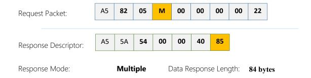
RPLIDAR will enter the measurement sampling mode once it receives the express scan(EXPRESS\_SCAN) request. Different from the scan(SCAN) request, this request will make RPLIDAR work at the sampling rate as high as it can be. For LIDARs support sampling more than 4000 times per second, the host system should use GET\_LIDAR\_CONF command to get "Typical Scan Mode", and use this command to make LIDAR work under its best performance and output measurement sample data accordingly.
