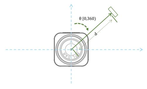
Figure 4-6 Angle and Distance Value Geometric Definition for RPLIDAR S1
